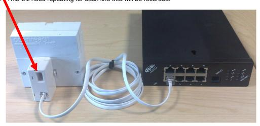
Should the cables that are provided not be suitable then the two wires provided by the carrier will need to be connected to pins 4 and 5 of an RJ45 socket that is connected to the front of the call recording unit.
