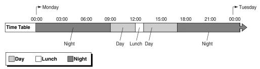
Note that time service modes can be arranged as they are needed (for example, night mode can occur in the morning and afternoon, if necessary) and not all time service modes need to be used in a time schedule. Also note that day mode or night mode resumes automatically when lunch mode ends.
